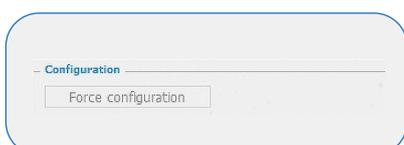
12 > The **Force Configuration** button allows to send the configuration command to the device via the BMeters wired peripheral (IR or NFC).
