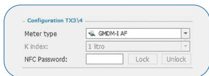
**1** > Where required, it is necessary to **select the type of meter** on which the radio module will be applied (in the example in the photo for the IWM-TX3/TX4 product). The **K index** is a non-modifiable field and represents the liters/rotation ratio. The **'NFC Password'** field allows to block/unblock the NFC side of communication via an 8 hexadecimal character password.
